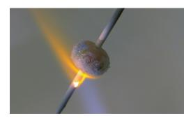
Carefully heat the bead in the very back of the flame, on the left, on the right, in the middle ...
