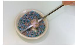
Start by heating the mandrel until the release agent starts to glow. Then make a base bead with CIM Gellys Sty and let it harden a little. Now heat the surface properly and roll it in frit – here we used the fritblend "Spring Blossoms" by Vetromagic. It doesn't have to be covered completely, but evenly. Melt the frit in and heat the bead until the frit start to spread.
