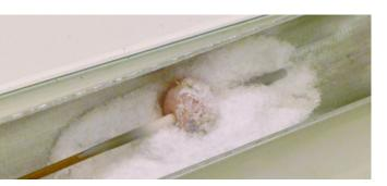
Heat the surface of the bead evenly and roll it quickly in glass powder "Morning Dew" by Vetromagic.
